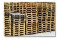
Load in stacks of no more than 15 pallets high Position the front of the load against a headboard or a braced loading rack
